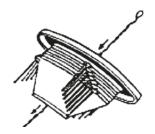
Grasp the trap's white lid and feed wire hanger through the center hole. Continue to draw hanger through the hole until it extends past the collapsed funnels.
