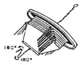
Bend the free end of the wire twice to form a Z shape. Bending the wire in the form of a Z ensures that the trap's weight does not "unbend" the wire, allowing the trap to fall.
